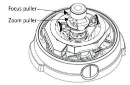
**Note:** The DC-Iris should always be disabled while focusing the camera. This opens the iris to its maximum, which gives the smallest depth of field and thus the best conditions for correct focusing. When the focus is set with this method it will then be maintained in any light conditions.
